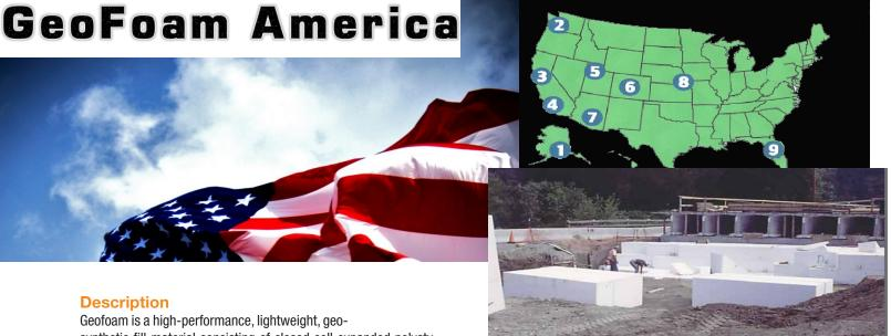
synthetic fill material consisting of closed cell expanded polystyrene (EPS). Geofoam is manufactured from to high-quality standards and meets or exceeds the requirements of ASTM D6817, Standard Specification for Rigid Cellular Polystyrene Geofoam. Geofoam is manufactured in a common density range between .70 to 2.85 lb/ft3 (11.2 - 45.7 kg/m3) and is an ideal, lightweight fill alternative for many construction applications.
